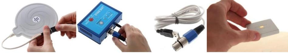
The field indicator in this mode glows brightly above the coil (Fig.), the intensity and range of the indicator depends on the power level set on the generator (output current).
