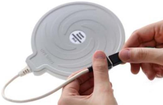
If the coil is connected to the generator **with a cable without color marking**, this is a **low-voltage capacitive mode**, if the connection is made with a **color marking cable**, then this is a **high-voltage capacitive mode** (in this case, the generator automatically switches to high-voltage mode and when the generator is turned on, a blue LED on its front panel lights up, for more details see section 2.4).
