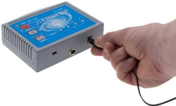
When power is applied, a short beep is heard, the LEDs on the front panel briefly light up and go out, which indicates that the generator goes into standby mode, in which it can be for an unlimited time.
