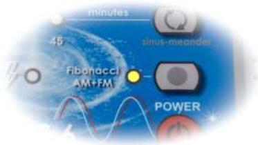
You can turn this modulation on or off with the middle button labeled “**Fibonacci AM + FM**” on the front panel of the generator. When “**Fibonacci AM + FM**” modulation is off, you can enable and configure fixed amplitude and / or frequency modulation via an external computer application, if necessary.
