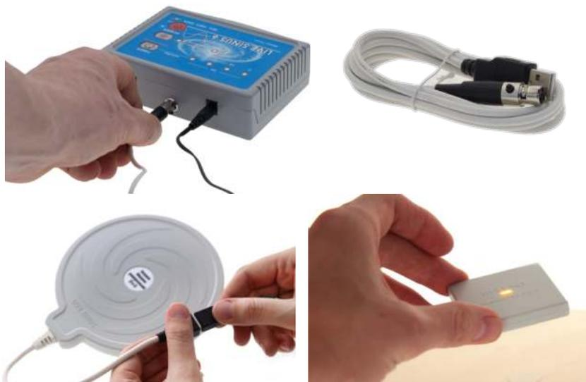
The electromagnetic field indicator (in a rectangular gray plastic case) in this mode glows brightly above the coil, the intensity and range of the indicator glow above the coil depends on the power level (output current) set on the generator.
